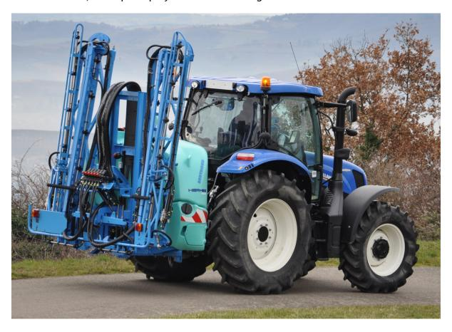
The new HERMES is available with a choice of 3 tank sizes: 800, 1000 and 1200 litres and a new range of ALSR rear-folding booms of 15, 16 or 18 metres. This new boom with 3 steel arms benefits from BERTHOUD's wealth of experience. Suspension on AXIALE central pivot system gives this boom excellent stability and good performance on slopes, turns and headlands. Robust and compact due to its "L" structure, it complies with the regulatory road width of 2.55 m.
