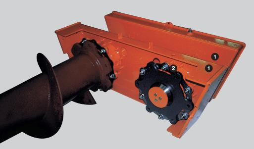
The EUROMIX II features a patented auger drive - FLEXIDRIVE - consisting of a series of gears and comprising a reversing system as standard. Each auger is connected to the drive via a gearbox.
