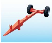
The body is assembled and welded in a swivel jig to obtain a constant quality finish and maximum rigidity to withstand impacts on loading.
